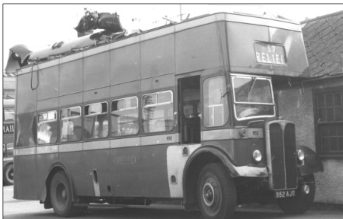
952 AJO, after its collision with Oxford station bridge
