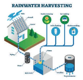
The illustration shows the principle of a rainwater harvesting system. The main tank can be above ground or underground, as required.
